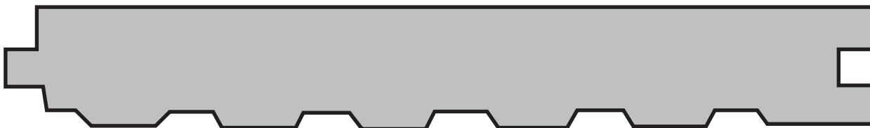
SP5 RW FLOORING OR PANELING
